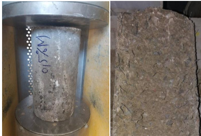
Figure 8: Test method and specimen failure with 0.5% fiber in the case of the compression test The results of the compressive and flexural strengths of the studied self compacting concretes are summarized in table 7.
