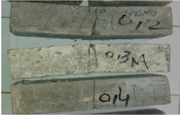
Figure 12: Ductile failure mode for SFRSCC1, SFRSCC2 and SFRSCC3.
