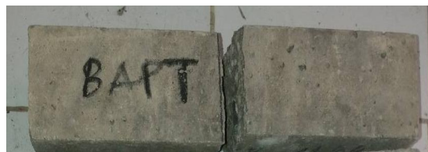
Figure 11: Failure of the control concrete (Brittle failure at mid-span).
