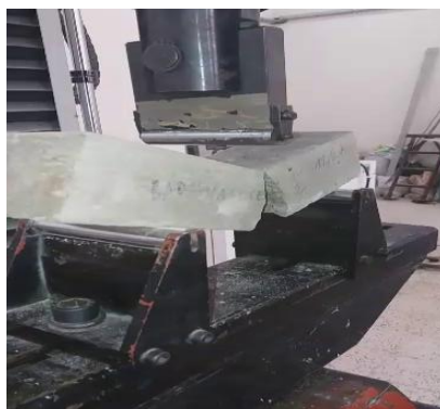
Figure 11: Failure of the control concrete (Brittle failure at mid-span).
