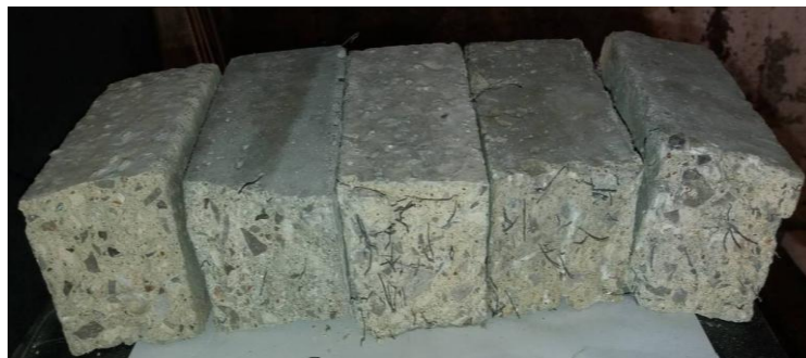
Figure 7: Distribution of fibers in the SCC specimens subjected to the bending test
