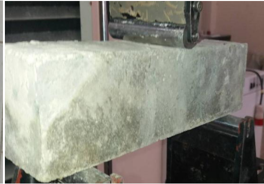
Figure 13: Densification of cracks and ductile failure for the case of SFRSCC4 (0.5% fibers).
