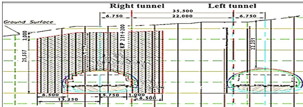
Figure 2: The extended of the section to treat
