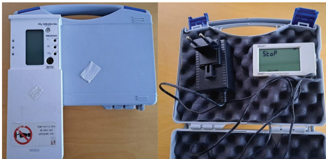
Fig. 2 Vaisala sensor on the HOBO data logger case
