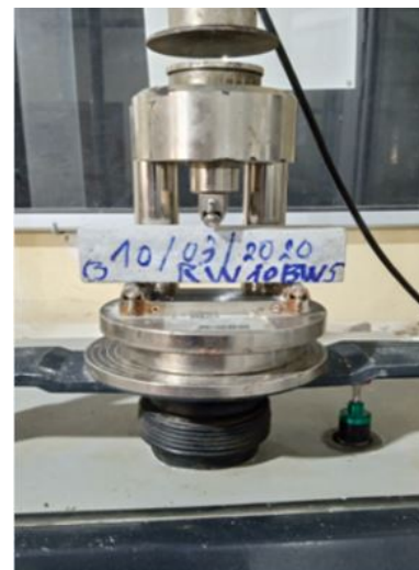
Fig. 5 The three-point bending flexural test on the 4 \times 4 \times 16 cm specimens
