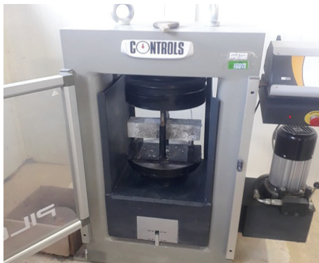
Fig. 3 Flexural strength test
