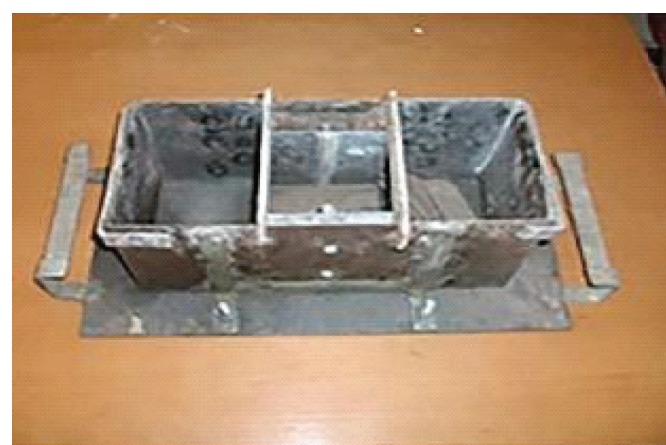
Fig. 8 Formwork for tensile specimens
