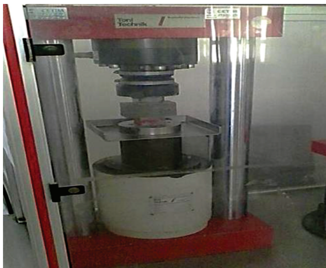
Fig. 3 Simple compression instrument
