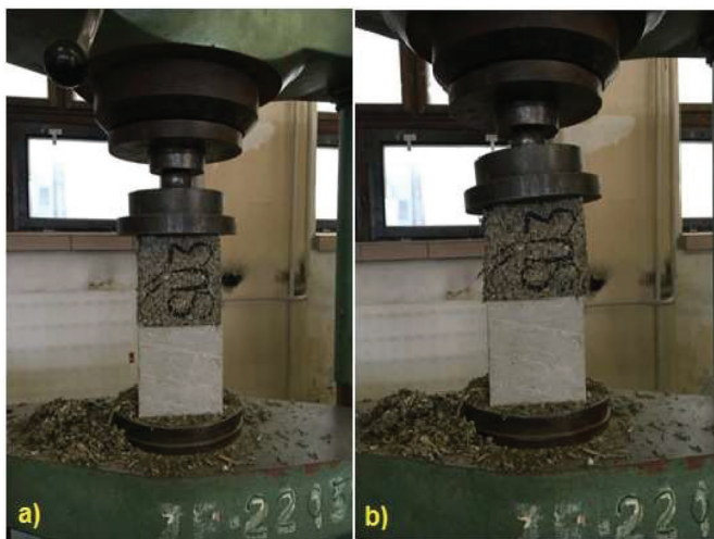
Fig. 5 Test sample stored in a hydraulic press: a) before loading; b) after loading.
