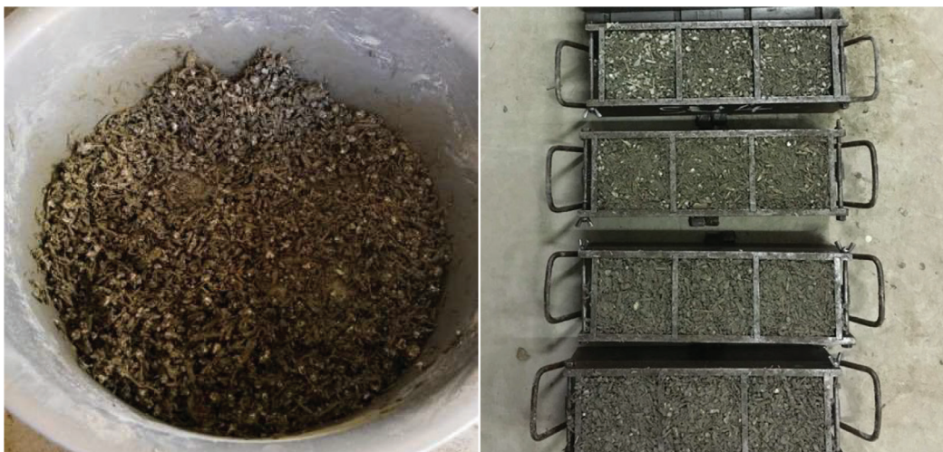
Fig. 2 The mixture of fresh concrete and moulds filled with the manufactured samples
