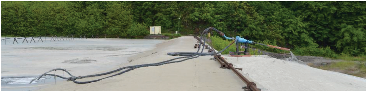
Fig. 5 Deposition of ore waste by the hydrocyclone
