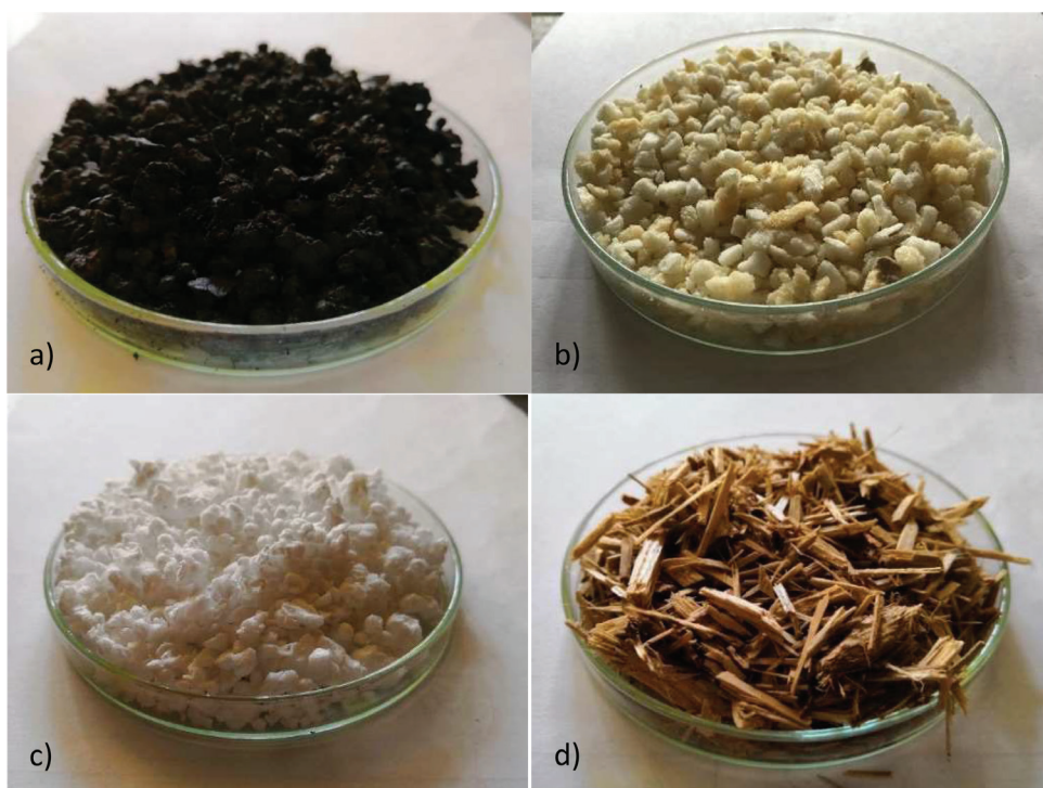
Fig. 1 a) Recycled polyethylene fraction 4/8 mm, b) Recyclate from waste polyurethane fraction 4/8 mm, c) Recycled from expanded polystyrene fraction 4/8 mm, d) Wood chip fraction 4/16
