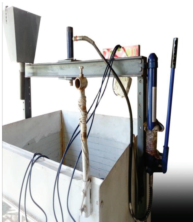
Fig. 1 Steel loading frame and hydraulic jack system.
