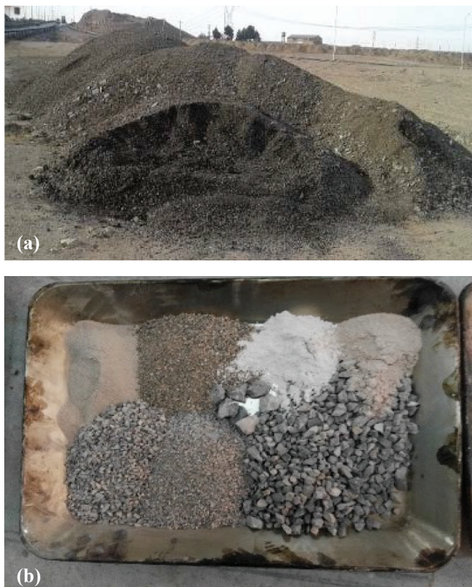
Fig. 2 (a) The location of the extraction of the crushed asphalt materials, (b) The appearance of the coarse-grained RAP after eliminating the bitumen.
