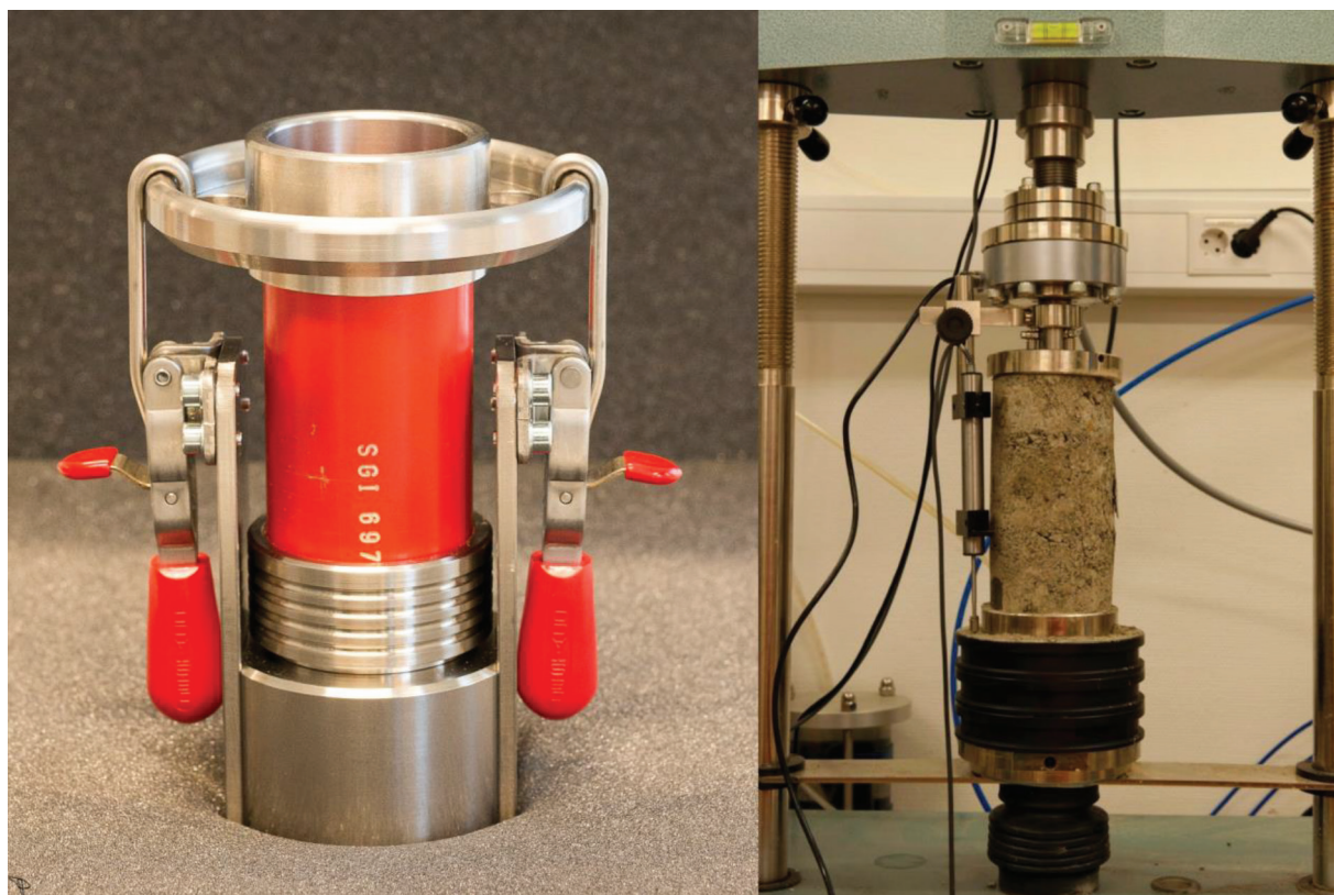
Fig. 1 Left: Photo showing packaging equipment for packing specimens with a height of 100 mm. Right: UCS testing apparatus showing a specimen after the UCS test. Photo source: Per Lindh
