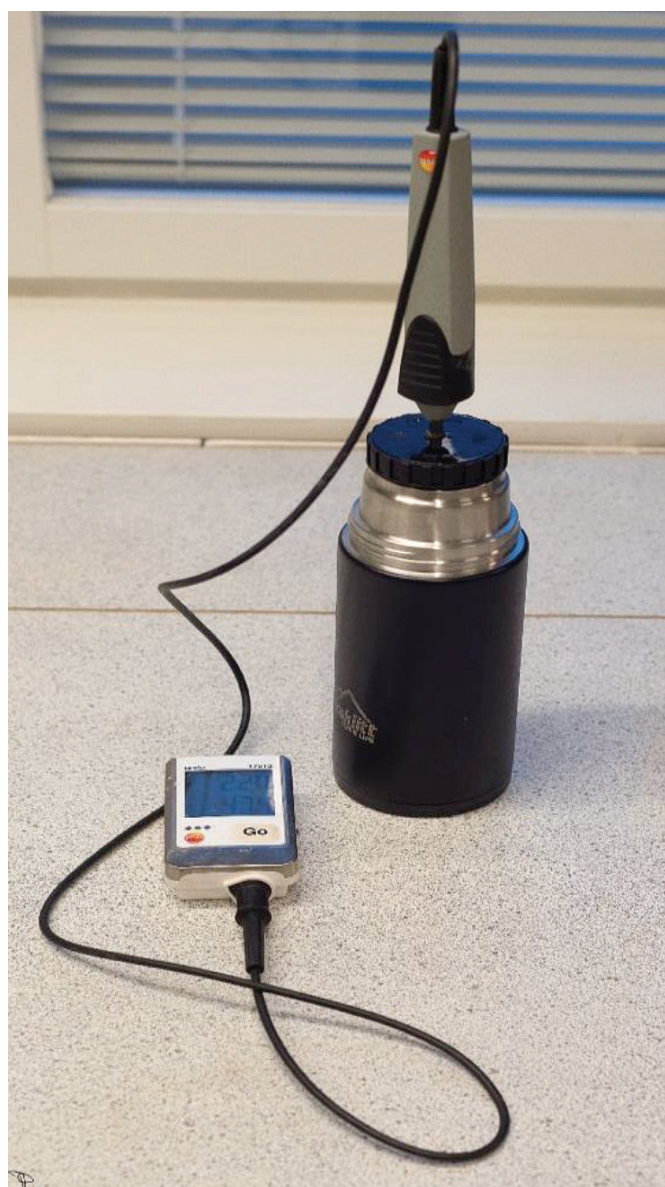
Fig. 4 Photo showing a simplified calorimeter consisting of a thermos and a temperature logger. Photo source: Per Lindh
