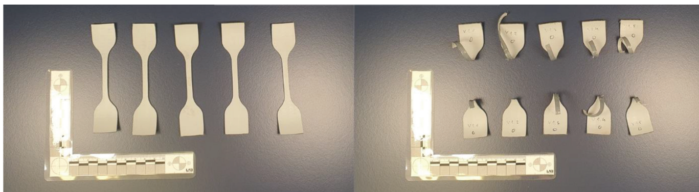
Fig. 11 Samples - photo before and after the strength test
