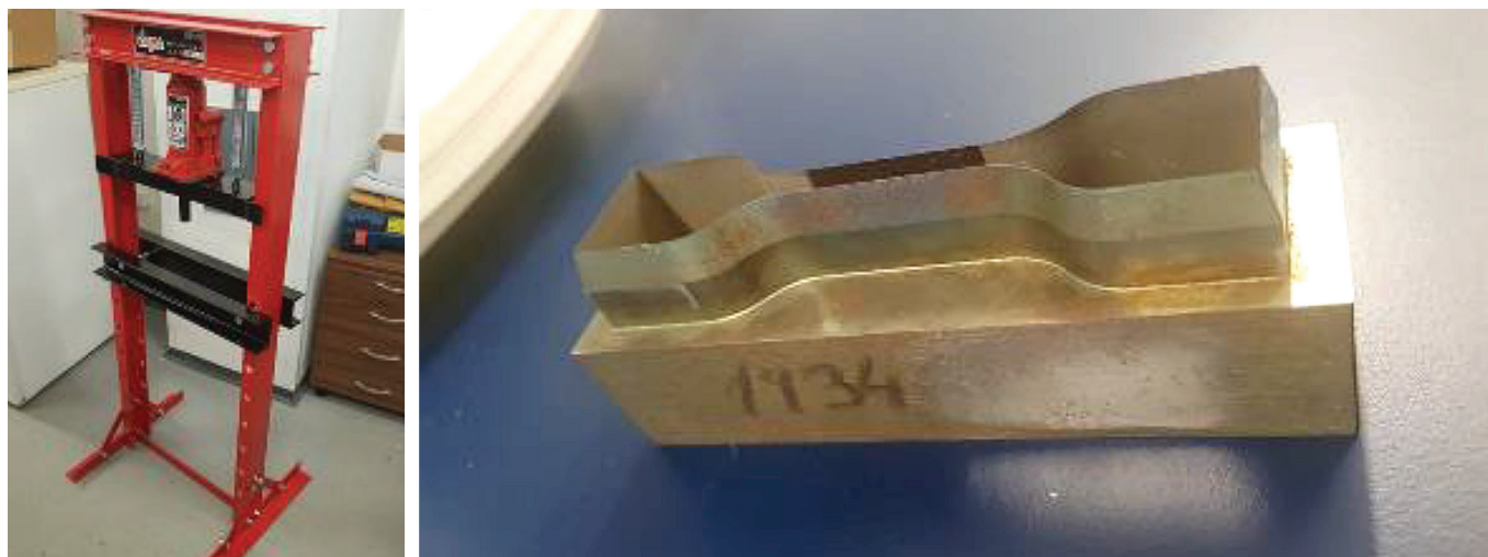
Fig. 6 Manual hydraulic press (left), steel punch (right)
