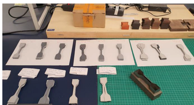
Fig. 10 Preparation of samples for the strength test
