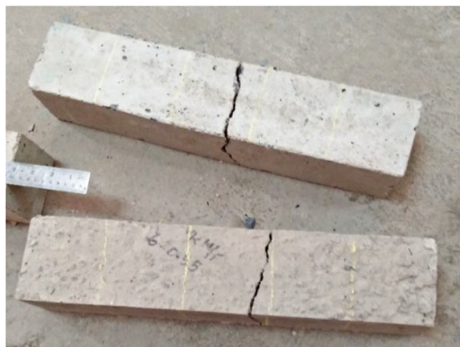
Fig. 6 Flexural strength failure of AAFGC
