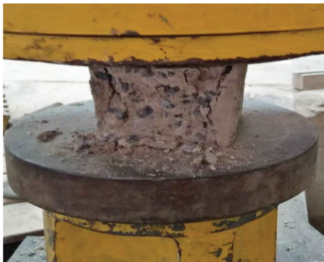
Fig. 4 Failure of AAFGC cubes
