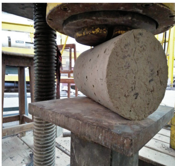
Fig 5. Split tensile failure of AAFGC
