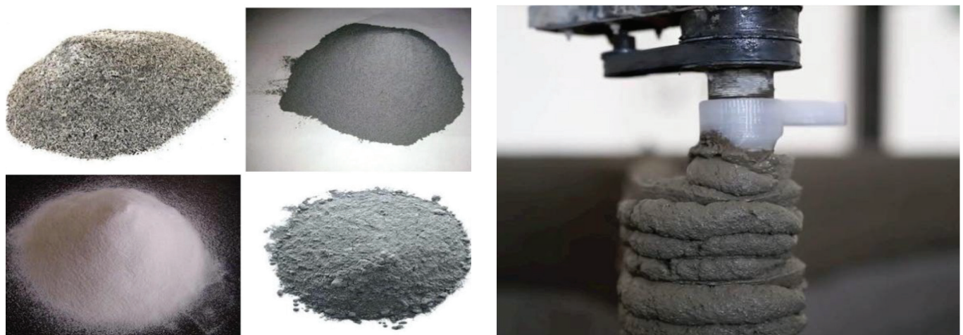
Fig. 5 Different types of additives (superplasticizers, viscosity modifiers, accelerators and retardants) for use in 3D printed materials, and a sample printing process after adding the retarding additive (Source: Mastercivilengineer, 2021, Digital manufacturing experts, 2020)
