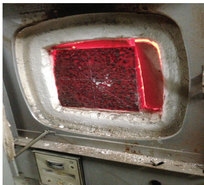
Fig. 5 General view of the furnace and the sample after one-sided heating in the inside of the furnace to a temperature of 1000 °C
