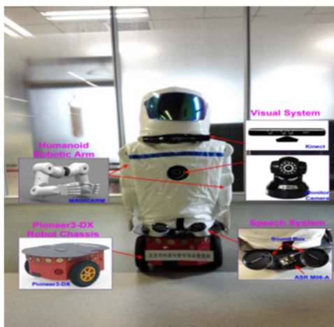
Figure 3 a) Structure of the robot [13]
