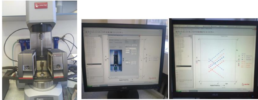
Figure 2. Dynamic shear rheometer Physica MCR301 (left), SW for the test and results (right)
