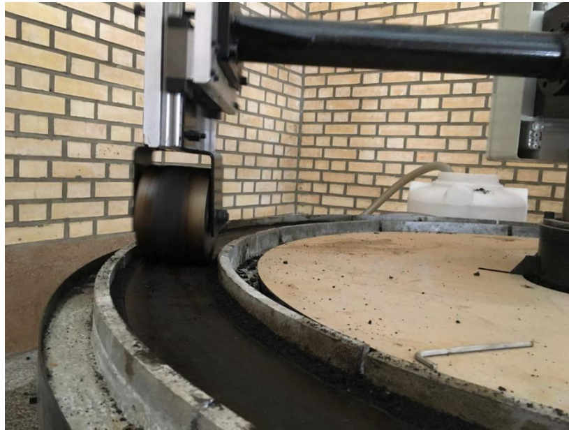
Figure 5. Asphalt mixture compaction
