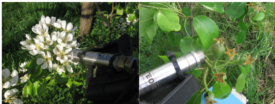
Fig. 1. Measurement of the surface temperature of plant tissues with an infrared sensor.
