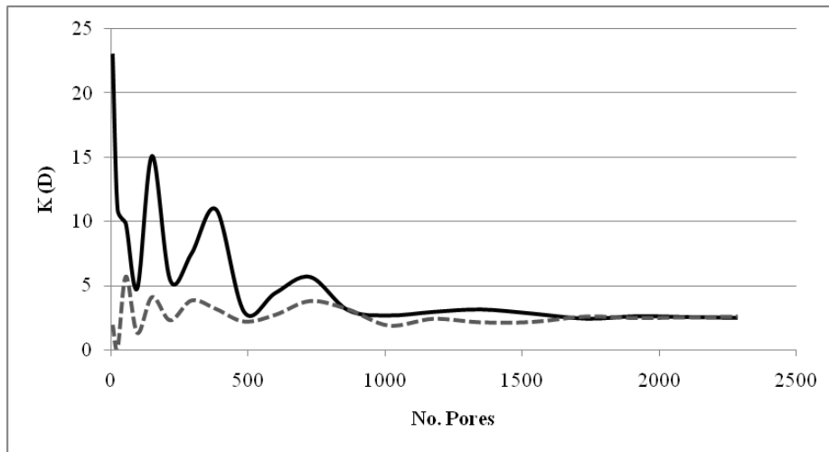
Figure 6. Effect of number of pores on absolute permeability.
