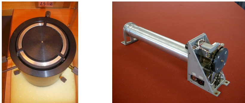
Figure 2. First space experiment with Czech grazing incidence X-ray optics was the X-ray telescope with photographic recording developed in collaboration with Poland and Soviet Union for the Vertikal 8 rocket flight in 1979. Left: The X-ray mirror. Right: The telescope.
