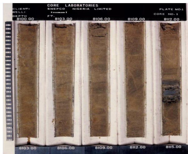
Fig.3. Core sample from FREEMAN 1 (8100-8111 ft).
