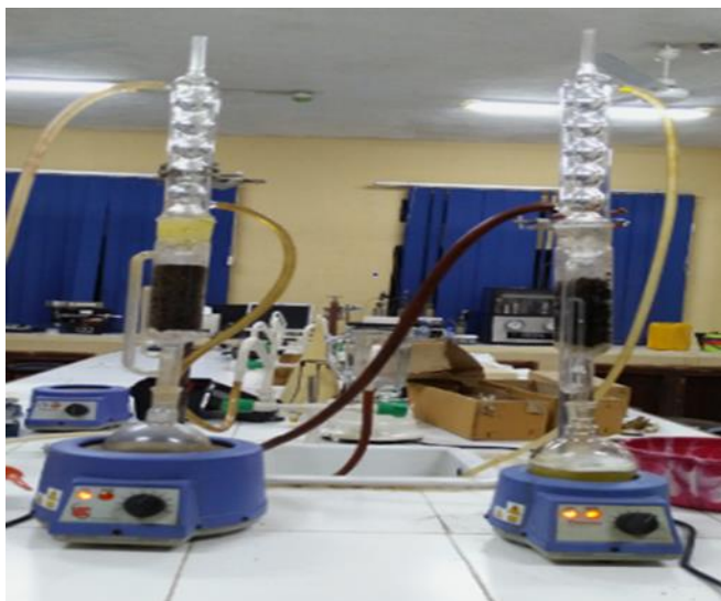
Figure 2. Setup of Soxhlet extraction for the pilot tests at Covenant University Petroleum Laboratory
