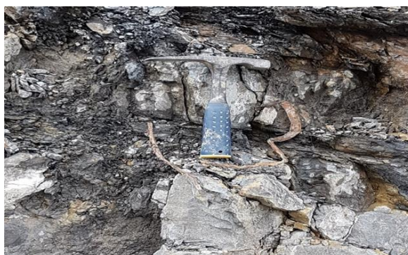
Fig. 14. Fault structure indicated by the alignment of shale and sandstone at the same depth from BEL-3 outcrop
