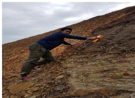
Figure 3. Spectral Gamma Ray (SGR) reading of the outcrop
