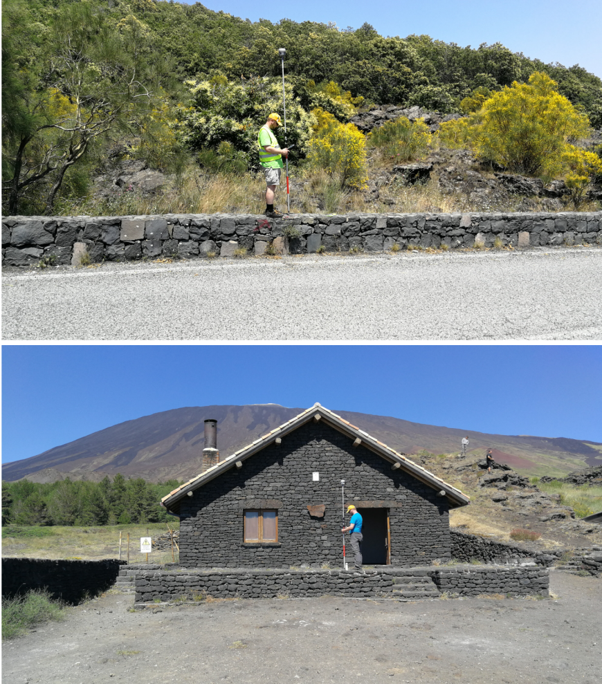
Fig. 5. GNNS measurements on one of relative benchmarks situated on the top of roadside rock-wall (top) and in the front of a refuge with an absolute gravity point inside (bottom).
