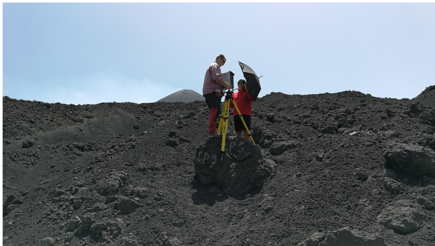
Fig. 6. Tower VGG measurement at point LZ (in its top position) in unusual conditions (with a view of NE creater in the background). Umbrella had to be used to shield the meter from wind.
