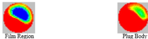
Figure 6. Film and plug unit at  $V_{so}=0.1$  m/s and  $V_{sg}=0.3$  m/s,  $\mu_l = 1000$  cP
