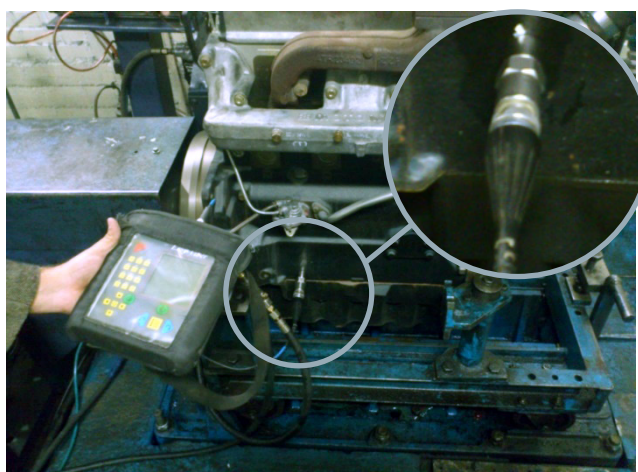
Fig. 4 Vibrometer connection to engine
