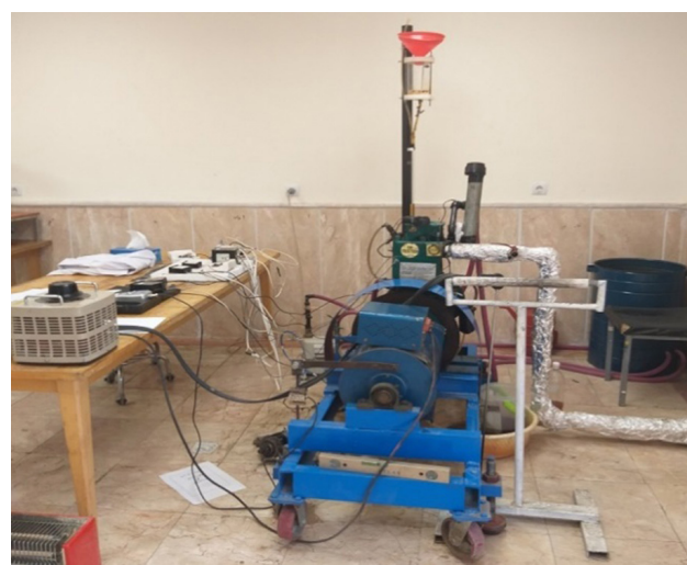
Fig. 1 Diesel engine test stand
