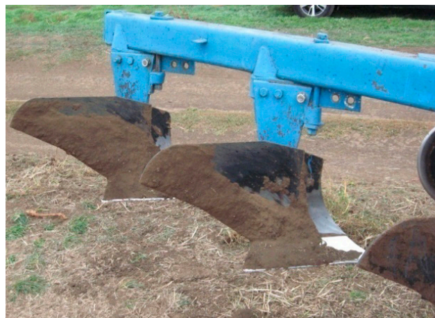
Fig. 5 Steel mouldboards with soil sticking
