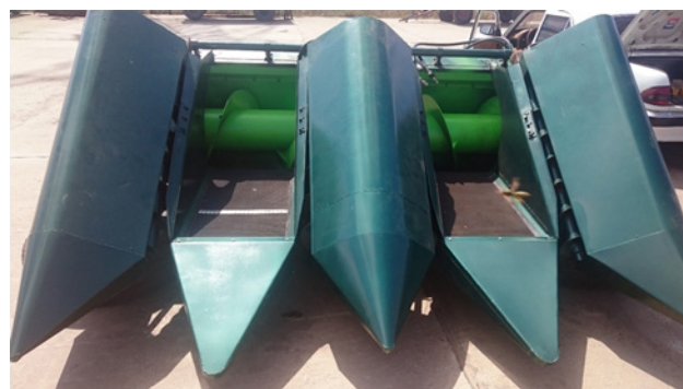
Fig. 2 The four-row header for Delta combine for sunflower harvesting
