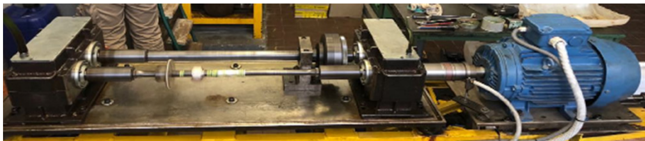
Fig. 1 Niemann M01 FZG back-to-back test rig
