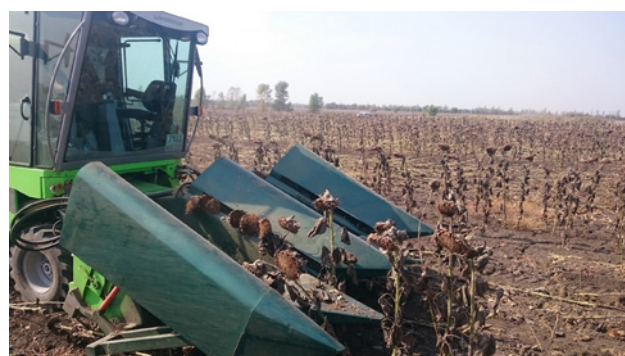
Fig. 3 Four-row header during harvesting of sunflower line VK-678B
