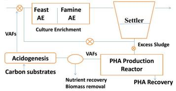
Figure 4 Aerobic Dynamic Feeding System
