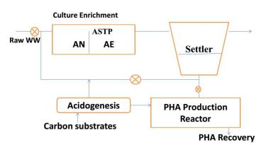
Figure 3 Anaerobic-aerobic Process
