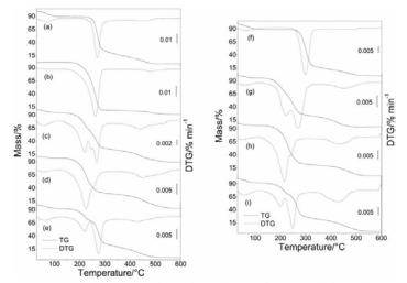
**Figure 1** TG/DTG curves of: regular maize starch (a), aceclofenac (b), (c) mixture aceclofenac:regular maize starch (2:1), (d) mixture aceclofenac:regular maize starch (1:1) and (e) mixture aceclofenac:regular maize starch (1:2), waxy maize starch (f), aceclofenac (b), (g) mixture aceclofenac:waxy maize starch (2:1), (h) mixture aceclofenac:waxy maize starch (1:1) and (i) mixture aceclofenac:waxy maize starch (1:2).
