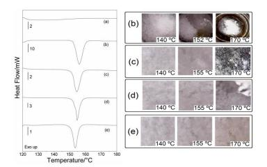
**Figure 2** DSC curves (left) and Thermomicroscopy (right): regular maize starch (a), aceclofenac (b), (c) mixture aceclofenac:regular maize starch (2:1), (d) mixture aceclofenac:regular maize starch (1:1) and (e) mixture aceclofenac:regular maize starch (1:2).
