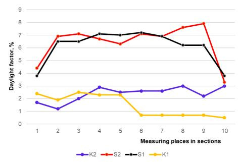
Figure 6 Daylight factor values in the reconstructed stable
