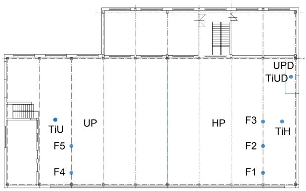
Figure 1 Scheme of measuring places in the mechanization and repair hall
