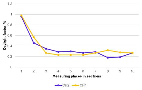
Figure 5 Daylight factor values in the original stable
