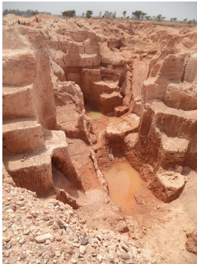
Fig. 16 Step bench work for Tin mining since the early 19th century being destroyed by artisanal activity (Goki et al., 2016)
