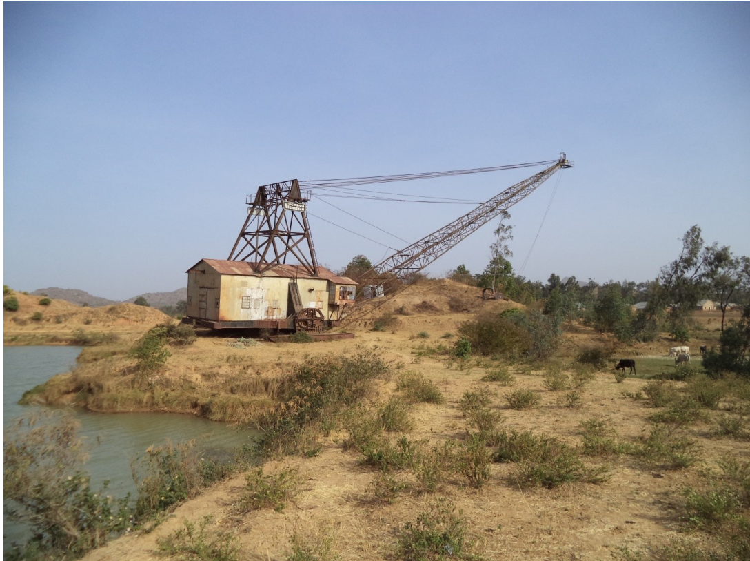
Fig. 13 Dragline used dated near a century used by the early tin miners on the Plateau
