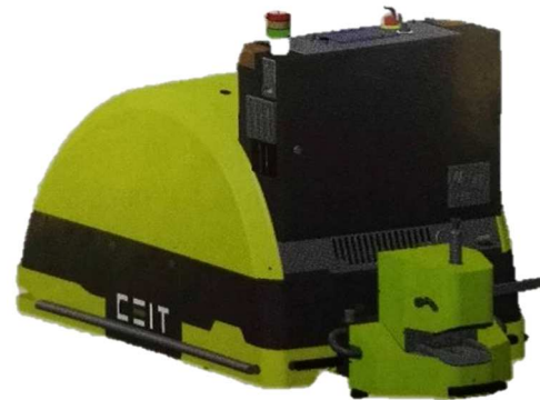
Figure 7 Automatic plug-in and disconnecting module with reverse module [13]
