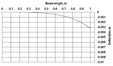
Figure 3 Deflection curve of the loaded beam form exact solution
