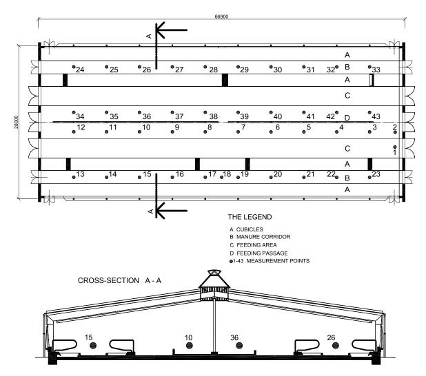
Figure 3 Ground plans and the cross-section of the measured building
