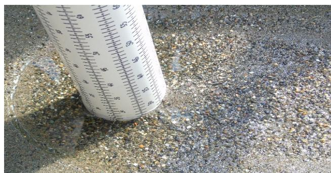
Fig. 3. Armour layer developed around the 17-cm-pier.
