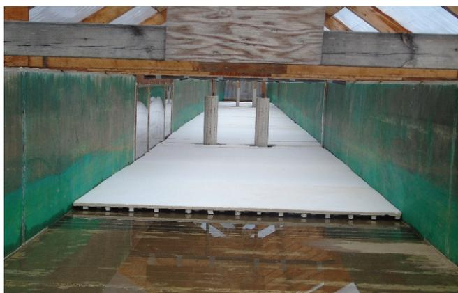
Fig. 2. Rough model ice cover on water surface.
