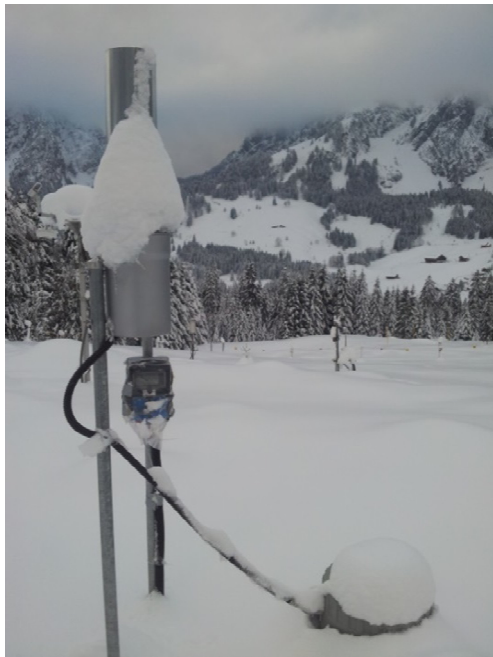
Fig. A3. Unheated precipitation collector with extended funnel connected to the 6712-Teledyne Isco automatic water sampler during the winter season 2015/16.
