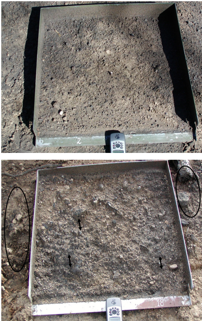
Fig. 4. Example plots from a) the burned 20% site, and b) the burned 60% site. The metal plot frames delineate the 0.5 m 2 plot area from which the runoff and sediment samples were taken. Black ovals on b) show the rocks and stumps on site which can indicate macropores and increased ponding, while arrows highlight the rougher soil surface texture which slows surface flow and may increase infiltration.
