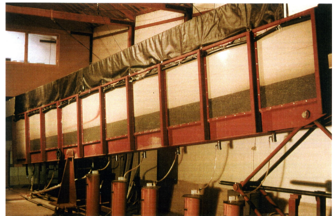
Fig. 1. A front view of the filled 10-m tipping trough (dark brown material = capillary block, light-colored material = capillary layer, and collection sump in the left-most segment). A dye tracer experiment with a red tracer is depicted on the left side. The irrigation system is inside the black box on the top of the tipping trough. Photo: Institute of Soil Science, University of Hamburg.
