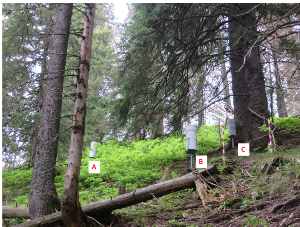
Fig. 2. Throughfall measurements in the mature spruce forest in the research plot Červenec: in the canopy gap „GAP“ (A), in the dripping zone at the crown periphery „CROWN“ (B) and in the central crown zone near the stem „STEM“ (C).
