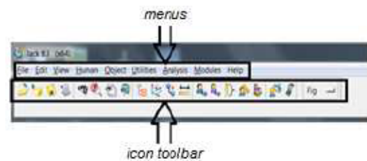
Figure 3 Control bar – Tecnomatix Jack
