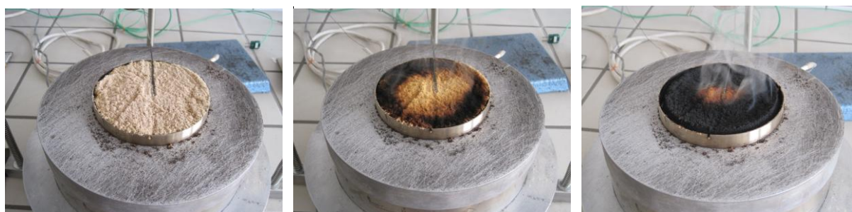
Fig. 2 Carbonization of dust sample during the testing
