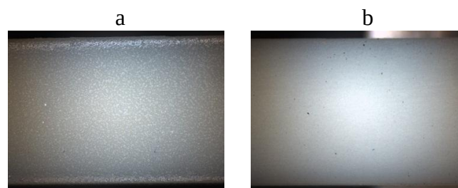
Fig. 4 Particle dispersion of the PTFE-particles in the matrix: a: 10 % PTFE, b: 40 % PTFE
