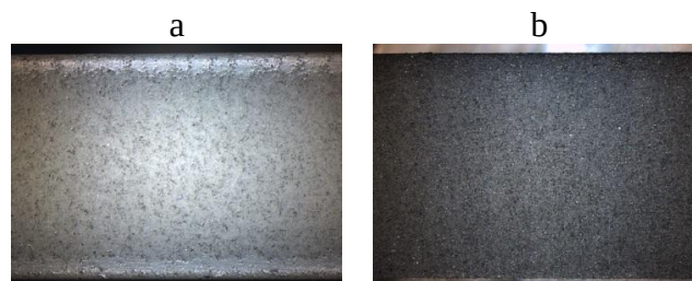
Fig. 5 Particle dispersion of the graphite-particles in the matrix: a: 10 % graphite, b: 40 % graphite
