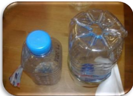
Fig. 5 Damage on the rectangular shaped bottle (own source)
