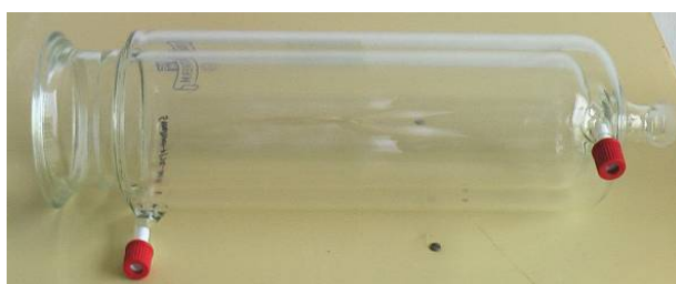
Fig. 5 Bioreactor, volume 3000 ml
