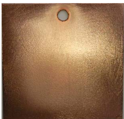
Fig. 3 Appearance of correct bright copper coated tin with bright coat using PV panels
