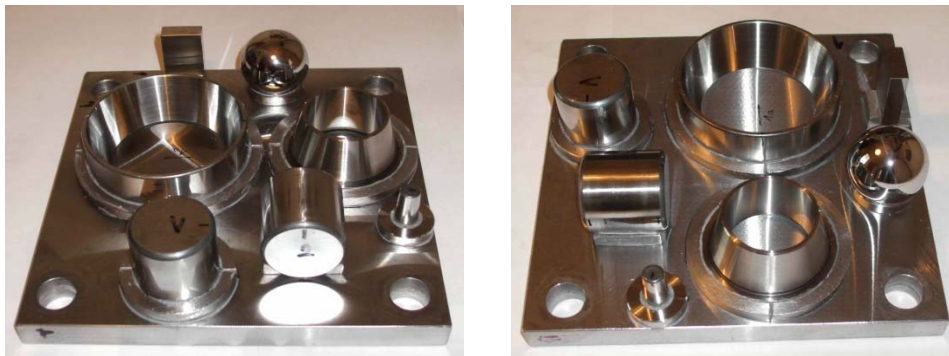
Fig. 7 Complex experimental artefact with high and known precision.
