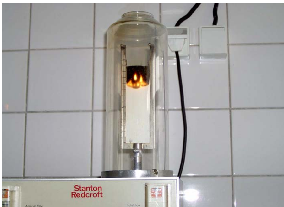
Fig. 8 Equipment of combustibility determination by the method of oxygen index (vertical modification)
