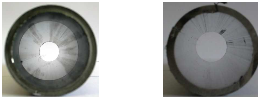
Fig. 2 Detail of the inner tubes' surface grade OR-3) \varnothing 55 \times 4.75 , first- draw, b) \varnothing 50 \times 3.75 , second- draw
