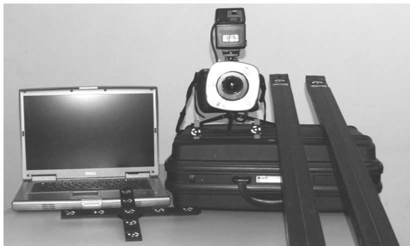
Fig. 2 Non-contact optical measuring system TRITOP
