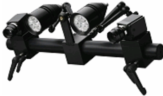
Fig. 1 Optical measuring system ARAMIS [4]
