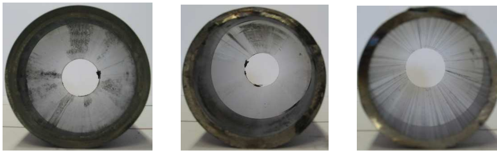
Fig. 1 Detail of the inner tubes' surface material E355 a) \varnothing 57 \times 5 , first- draw, b) \varnothing 50 \times 3.75 , second- draw c) \varnothing 44 \times 3 , third- draw
