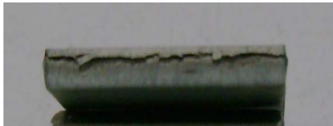
Fig. 2. The crack shape at 180^{\circ} bend test (CP-W 800)
