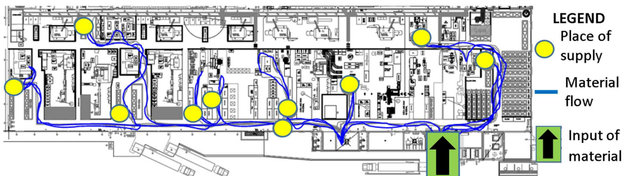
Figure 1 Flow of material in the current state of supply Source: Internal document of company, edited by author
