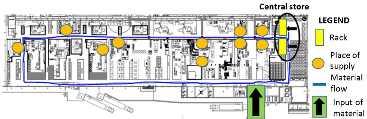
Figure 2 Visualization of material flow with new supply points
