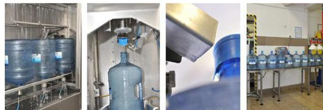
Figure 2 Process of the filling, cleaning, labelling and preparation of the water for the distribution
