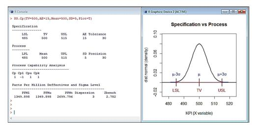
Figure 1 – Output of Function SS.Cp, Comparing a Process with  $\mu$  Adjusted to TV, and with  $\sigma$  = AE/3. The Dispersion is 3, Cp = CpK = 1 and 2700 PPM are Produced, Corresponding to a Z<sub>bench</sub> = 2.78. The Process Parameters  $\mu$  and  $\sigma$  are not Calculated, but Stipulated by the User
