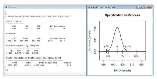
Figure 2 – Output of Function SS.Cp, Showing a Process with a 1.5 $\sigma$  Shift to the Left of the TV, with  $\sigma$  = AE/4. The Dispersion is 4, Cp = 1.33, Cp<sub>K</sub> = -0.833 and 6200 PPM are Produced, leading to a Z<sub>bench</sub> = 2.5
