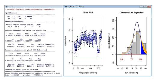
Figure 3 – Output of Function SS.Norm, Showing a Real Industrial process dealing with Daily Losses in Juice Production. The Process has Very Low Performance (Pp = 0.62) and is Displaced towards the Right ( $Pp_K = 0.268$ ), Producing 108743 PPM Corresponding to a Long Term Sigma Level of 0.798. There are Evident Special Causes of Variation ( $p = 4.773959 \times 10^{-15}$ ), and a Cp = 0.95 Shows a Need for Improvement
