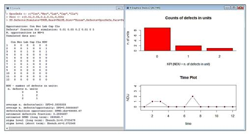
Figure 6 – Output of Function SS.Defects, in the Simulation Mode. Simulated Data is Presented on the Left-Hand Side, Together with the Main Metrics: DPU, DPO, DPMO and Sigma-Levels. On the Right-Hand Side, Barplot with Main Observed Counts of Samples per Number of Defects, and Evolution with Time. Z<sub>bench(LT)</sub> is Very Small and Z<sub>bench (ST)</sub> Must be Seen with Caution Since Its Meaning is Doubtful
