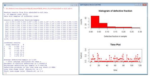
Figure 5 – Output of Function SS.Defectives, Showing a Real Industrial Process, Analysing Samples of Different Sizes of Pre-Packaged Coffee Beans. Units with Contents Lower than the Legal AE or Higher than the Internal AE, Are Defective. Z<sub>bench (LT)</sub> Shows Possibilities for Improvement
