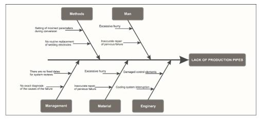
Figure 5 – Cause and Effect Analysis of Welding Electrode Failures
