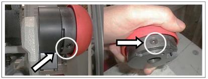
Figure 2 – Fixing Screw on Device
