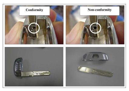
Figure 1 – Visualization of Missing Pin
