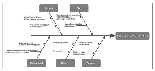
Figure 4 – Cause and Effect Analysis of Downtimes Due to Lack of Production Pipes
