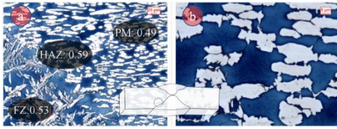
Fig. 9 Microstructure and ferrite proportion in different zones of the weld (a) and micrograph of the HAZ (b)
