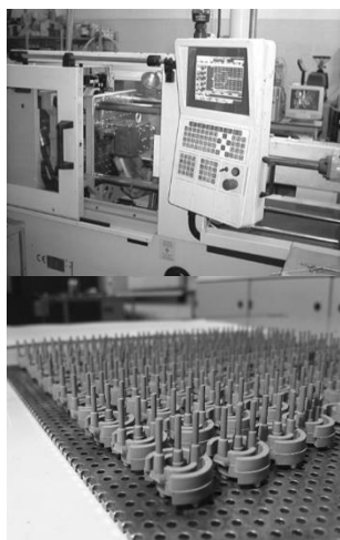
Fig. 10 Left: injection moulding press; right: moulded MIM parts placed on trays
