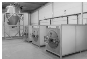
Fig. 11 Left: catalytic debinding furnace (courtesy Nabertherm GmbH); right: solvent debinding units (courtesy Lömi GmbH)
