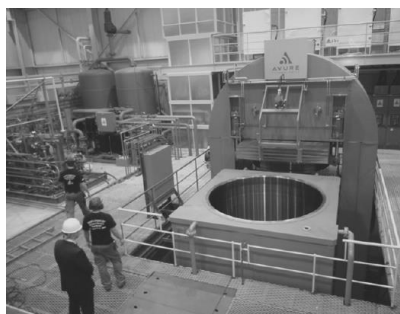
Fig. 15 Large-scale HIP unit (courtesy MTC/Avure)
