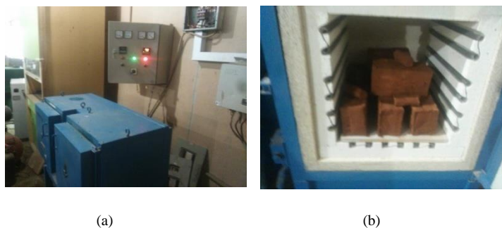
Fig. 1 Pictures of (a) electric furnace used in firing and (b) bricks samples
