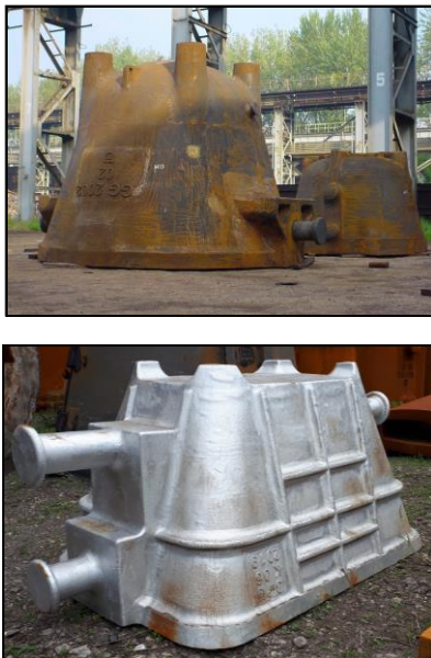
Fig. 1 Examples of slag ladles produced in Krakodlew S.A.
