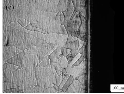
Fig. 1 The cross-sectional microstructures of specimens nitrided at 565°C for different time (a) 60min (b) 90min (c) 120min (d) 150min (e) 180min
