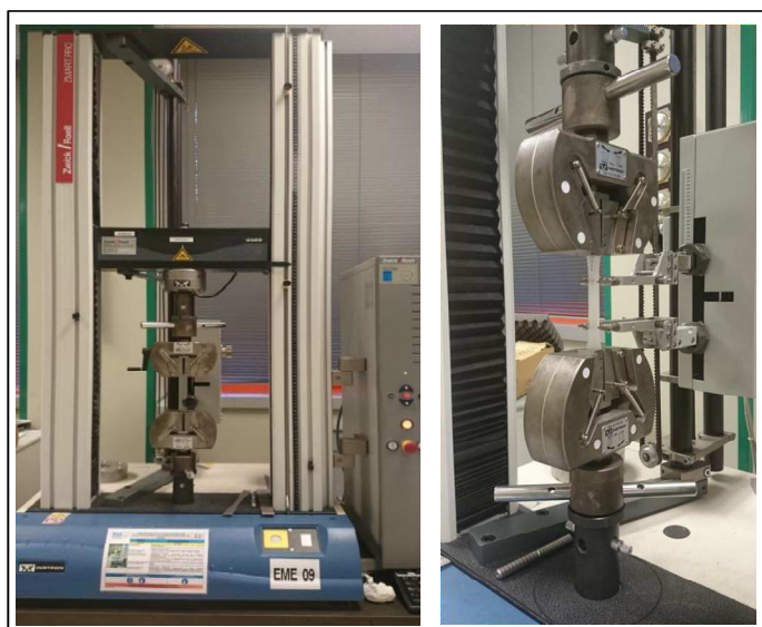
Figure 4 – Machine Used for the Tensile Test
